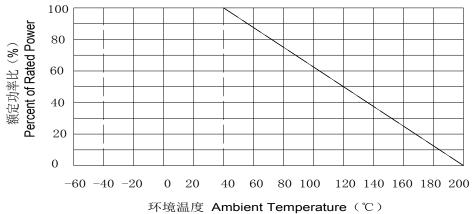
For resistors operated at the ambient temperature of 40°C or higher ,the power rating shall be derated in accordance with the above derating curve.
